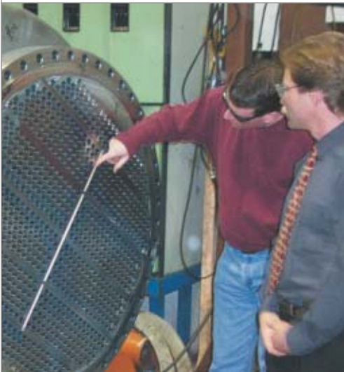
Ellett's David Clift (right) says that "everything had to be perfect" in fabricating the atypical heat exchanger. The tube holes [pointed out by Jim Hunt (left)] were drilled to tight tolerances.
